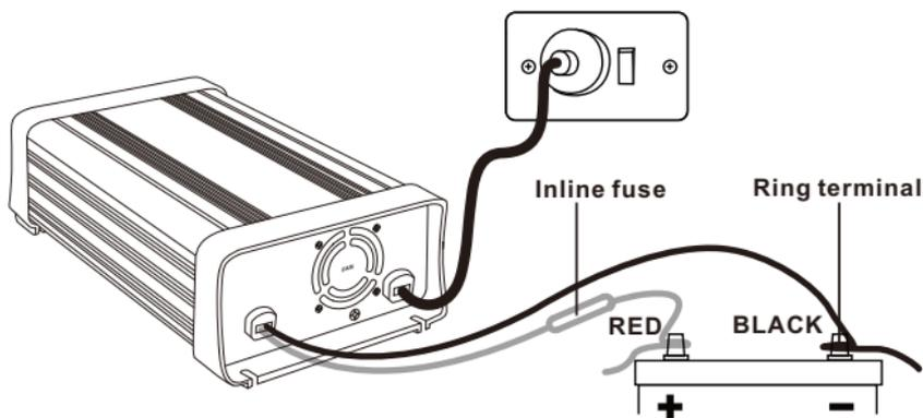
7. Fit the correctly rated fuse.
